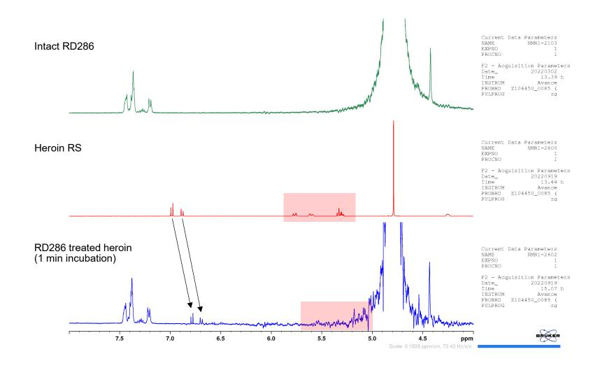
Figure 3. Comparative analysis of the  $^{1}H$  NMR spectra (3.8 – 0.7 ppm) of the intact RD286, the heroin reference standard, and the RD286 treated heroin sample.
